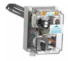
Single-stage immersion heaters are equipped with a three-pole control thermostat. When powered on, the heater will always operate at full capacity. Two-stage immersion heaters have a four-pole thermostat, and the heater operates in two stages (at partial capacity or at full capacity).
